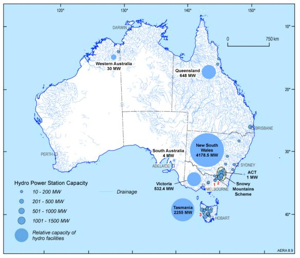
Figure 8.9 Major Australian operating hydro electric facilities with capacity of greater than 10 MW. Numbers indicate sites referred to in section 8.4.2 **Source:** Geoscience Australia
